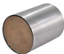
SUB51 Diameter= 110mm Length= 130mm Euro5 / 200cps (Cells) High Loading / Premium Quality
