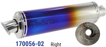
170056-02 Right 170056-02L Left S/Steel 304 / Titanium body "Twister" Perforated pipe Body Length = 435mm Inlet Diameter = 54mm Body Diameter = 122x97mm
