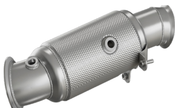
90812010 Diameter = 80/89mm Metallic Catalyst 300cpsi (Cells) BMW M135i - 435i / M2 (N55 - 3.0 - Euro 5/6)
