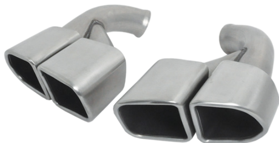
TR-3696 Left & Right S/Steel 304 / Brushed Polished Slant Cut & Side Slant Cut Porsche Cayenne Turbo '15-'16 Total Length= 440mm Dimensions= 200x100mm Inlet(OD)= 68mm
