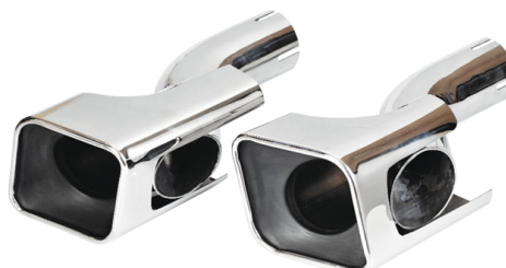
TR-3648 Left & Right S/Steel 304 Slant Cut & Side Slant Fits: Range Rover Diesel 2005-2013 "Range Rover Autobiography" Look Fits all Range Rover SPORT Diesel models with the Autobiography rear bumper Total Length= 310mm Dimensions= 120x115mm Inlet(ID)= 60mm
