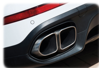
TR-3697 Left & Right S/Steel 304 / Brushed Polished Slant Cut & Side Slant Cut Porsche Cayenne 9YA Turbo '17- Total Length= 360mm Outlet Diameter= 2x102mm Inlet(ID)= 60mm
