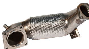
90813000 Inlet Diameter = 70/89mm Metallic Catalyst 300cpsi (Cells) Hyundai i30N / Performance (Euro 6)
