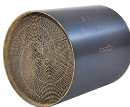
90603247 Diameter= 108mm Length= 100mm Euro4 / 200cpsi (Cells) HF+ (For High Temperature)
