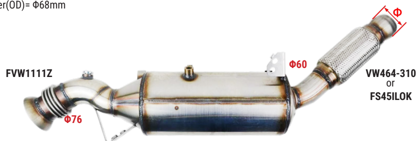
FS45ILOK Repair Flexible for Mercedes Spinter Total Length= 245mm Inlet Diameter(ID)= \Phi 60mm Head Diameter(OD)= \Phi 68mm
