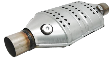
LFC502 Inlet Pipe Diameter= 60mm Body Dimensions= 180x110mm Length without ending tubes= 360mm Ceramic Substrate Euro5 High Loading 400cps / For engines up to 4.0 L
