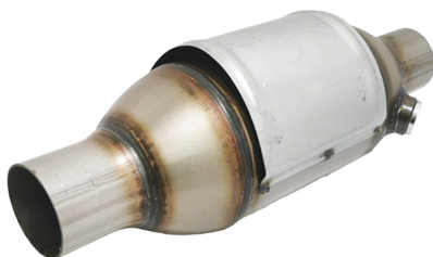
LFC603 Inlet Pipe Diameter= 60mm Body Diameter= 130mm Length without ending tubes = 230mm Ceramic Substrate Euro6 High Loading 400cps / For engines up to 3.0 L
