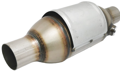
LFC303 Inlet Pipe Diameter= 60mm Body Diameter= 130mm Length without ending tubes = 230mm Ceramic Substrate Euro3 High Loading 400cps / For engines up to 3.0 L
