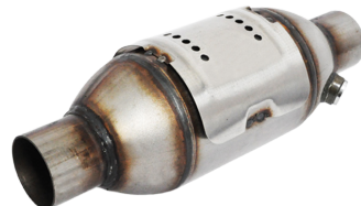
LFC601 Inlet Pipe Diameter= 50mm Body Diameter= 101mm Length without ending tubes= 220mm Ceramic Substrate Euro6 High Loading 400cps / For engines up to 1.6 L
