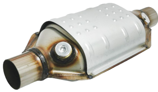
LFC500 Inlet Pipe Diameter= 50mm Body Dimensions= 150x95mm Length without ending tubes= 280mm Ceramic Substrate Euro5 High Loading 400cps / For engines up to 2.0 L
