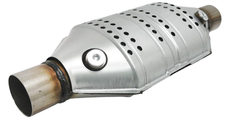
LFC302 Inlet Pipe Diameter= 60mm Body Dimensions= 180x110mm Length without ending tubes= 360mm Ceramic Substrate Euro3 High Loading 400cps / For engines up to 4.0 L
