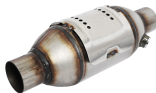
LFC401 Inlet Pipe Diameter= 50mm Body Diameter= 101mm Length without ending tubes= 220mm Ceramic Substrate Euro4 High Loading 400cps / For engines up to 1.6 L
