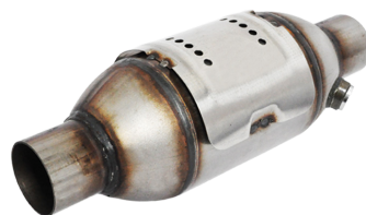
LFC604 Inlet Pipe Diameter= 54mm Body Diameter= 114mm Length without ending tubes = 220mm Ceramic Substrate Euro6 High Loading 400cps / For engines up to 2.0 L
