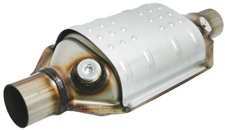
LFC400 Inlet Pipe Diameter= 50mm Body Dimensions= 150x95mm Length without ending tubes= 280mm Ceramic Substrate Euro4 High Loading 400cps / For engines up to 2.0 L
