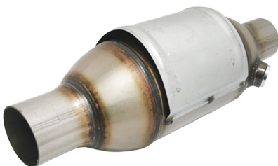
LFC403 Inlet Pipe Diameter= 60mm Body Diameter= 130mm Length without ending tubes = 230mm Ceramic Substrate Euro4 High Loading 400cps / For engines up to 3.0 L
