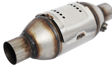
LFC304 Inlet Pipe Diameter= 54mm Body Diameter= 114mm Length without ending tubes = 220mm Ceramic Substrate Euro3 High Loading 400cps / For engines up to 2.0 L
