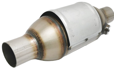
LFC503 Inlet Pipe Diameter= 60mm Body Diameter= 130mm Length without ending tubes = 230mm Ceramic Substrate Euro5 High Loading 400cps / For engines up to 3.0 L
