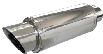
170262 S/Steel 304 "Rossi" style Body Length = 250mm Inlet Diameter = 60mm Body Diameter = 115mm With DB Killer TD=89mm
