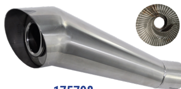
175798 S/Steel 304 "Twister" Perforated pipe Body Length = 300mm Inlet Diameter = 50mm Body Diameter = 100mm
