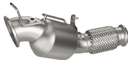
90822075 Diameter = 76/89mm Metallic Catalyst 200cpsi(Cells) BMW 20i / 30i / Toyota Supra (B48 - 2.0 - Euro 6d / 6d-Temp. - GPF)
