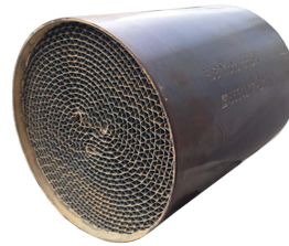
90603205 Diameter= 108mm Length= 130mm 100cpsi(Cells) PE (Perforated Foil to reduce weight & Backpressure)
