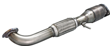
90814015 Diameter = 70mm Metallic Catalyst 200cpsi (Cells) Opel Astra J GTC (2.0 - Euro 5)
