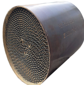
90603242 Diameter = 120mm Length = 100mm 100cpsi(Cells) PE (Perforated Foil to reduce weight & Backpressure)
