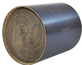
90603247 Diameter= 108mm Length= 100mm Euro4 / 200cpsi (Cells) HF+ (For High Temperature)
