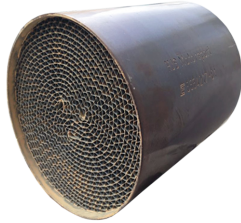
90603204 Diameter= 108mm Length= 100mm 100cpsi(Cells) PE (Perforated Foil to reduce weight & Backpressure)
