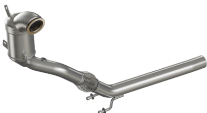
90951120 Diameter = 60mm Metallic Catalyst 200cps (Cells) Audi A3 III / Seat Leon III / Skoda Octavia III / VW Golf VII (1.2 / 1.4 - Euro 5/6)
