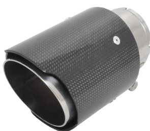
S/Steel 304 / Carbon / Double Layer / Slant Cut A070 Total Length= 165mm Outlet Diameter= \Phi 89 Inlet(ID)= \Phi 60
