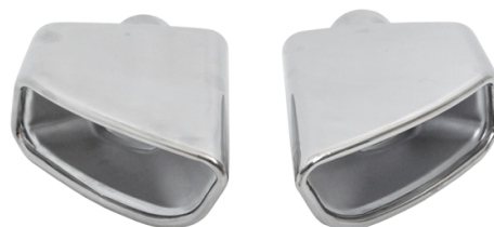
TR-3616A Left & Right S/Steel 304 Slant Cut & Side Slant Cut "BMW X6 V8 Look" Total Length= 320mm Outlet Dimensions= 210x85mm Inlet(OD)= 64mm
