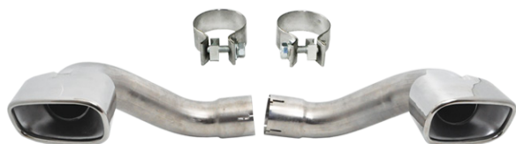
TR-3629 Left & Right S/Steel 304 Slant Cut & Side Slant Cut BMW X5 3.0 E70 2007-2010 "V8 Look" Total Length=350mm Outlet Dimensions=140x75mm Inlet(ID)=66mm
