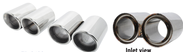
TR-3608 Left & Right S/Steel 304 Slant cut / Double Layer Total Length= 145mm Outlet Diameter= 2x89mm Inlet(OD)= 2x64mm
