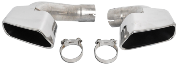
TR-3671 Left & Right S/Steel 304 Slant Cut & Side Slant Cut BMW X5 F15 2014-2017 M-Sport Style Total Length = 380mm(Left) & 300mm (Right) Dimensions = 185x75mm Inlet(ID) = 70mm
