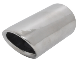
A039 Silver B039 Blue (Burned) M039 Black S/Steel 304 / Slant Cut VW Golf/Passat, AUDI Total Length = 145mm Outlet Dimensions = 70mm Inlet(ID)= \Phi 57 mm With Special clips which lock on the OEM tailpipes No welding needed
