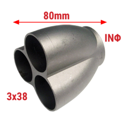
270131 3x38 IN50(OD) 270149 3x38 IN60(OD) 3-1 S/S Casting connector Fits on 3 pipes Φ38 each
