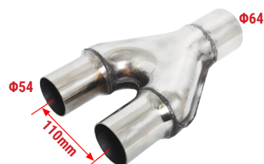
Y-PIPE-6051 Length = 260mm INΦ64 OUTΦ54 S/Steel Y-pipe
