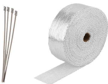
ALW-50 50mm Thickness=1.5mm / Length=9M Heat resistance: 550 °C Includes 4 Stainless Steel Tie Straps
