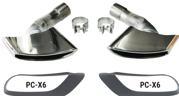
TR-3616 Left & Right S/Steel 304 Slant Cut & Side Slant Cut For BMW X6 E71 3.0idx 3.5idx 3.5ix 4.0d to give an 5.0i/ M50d V8 Look with 2 Plastic Cover Trims PC-X6 Total Length= 410mm Outlet Dimensions= 210x85mm Inlet(ID)= 67mm
