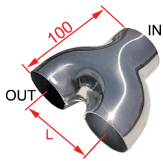
Y1 L=80 INΦ=58 OUTΦ=52 Y2 L=102 INΦ=58 OUTΦ=58 S/Steel Y-pipe
