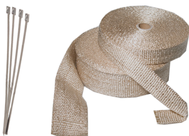
WHT1000-3 30mm WHT1000-5 50mm Thickness =1.5mm / Length=15M Heat resistance: 550 °C Includes 4 Stainless Steel Tie Straps
