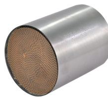
SUB52 Diameter= 120mm Length= 130mm Euro6 / 200cpsi (Cells) High Loading / Premium Quality
