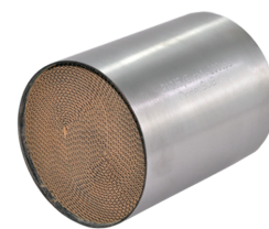
SUB63 Diameter= 130mm Length= 130mm Euro6 / 200cpsi (Cells) High Loading / Premium Quality
