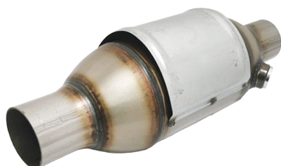
LFC303 Inlet Pipe Diameter= 60mm Body Diameter= 130mm Length without ending tubes = 230mm Ceramic Substrate Euro3 High Loading 400cps / For engines up to 3.0 L
