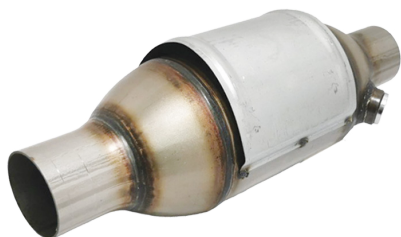
LFC403 Inlet Pipe Diameter= 60mm Body Diameter= 130mm Length without ending tubes = 230mm Ceramic Substrate Euro4 High Loading 400cps / For engines up to 3.0 L
