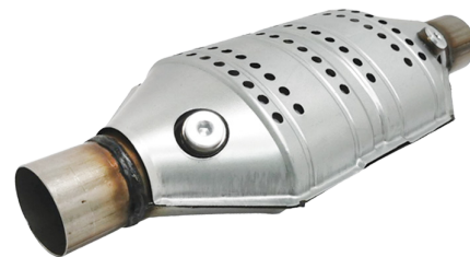
LFC302 Inlet Pipe Diameter= 60mm Body Dimensions= 180x110mm Length without ending tubes= 360mm Ceramic Substrate Euro3 High Loading 400cps / For engines up to 4.0 L
