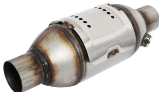
LFC301 Inlet Pipe Diameter= 50mm Body Diameter= 101mm Length without ending tubes= 220mm Ceramic Substrate Euro3 High Loading 400cps / For engines up to 1.6 L
