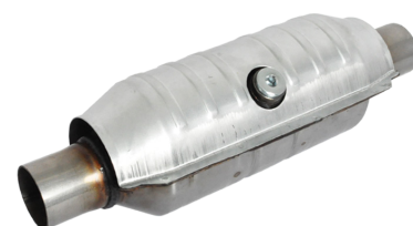
LFC410 Inlet Pipe Diameter= 50mm Body Diameter= 101mm Length without ending tubes = 290mm Ceramic Substrate Euro4 High Loading 400cps / For engines up to 2.0 L
