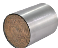
SUB40 Diameter= 100mm Length= 130mm Euro4 / 200cpsi (Cells) High Loading / Premium Quality
