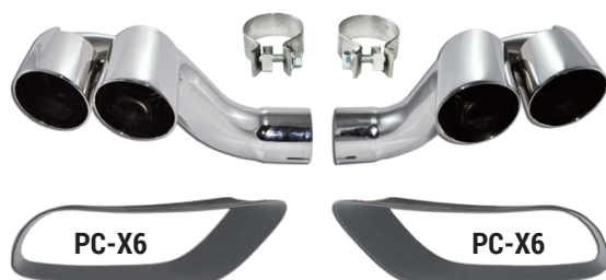
151991 Left & Right S/Steel 304 - Chrome plated BMW X6 E71 to give an M Look with 2 Plastic Cover Trims PC-X6 Diameter= 2x 80mm Inlet (ID)= 67-60mm
