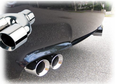
06-7720SL Left 06-7720SR Right S/Steel 304 / Chrome plated Slant Cut & Side Slant Cut Ferrari style Total Length= 225-185mm Outlet Dimensions= 2x76mm Inlet(OD)= \Phi 60mm
