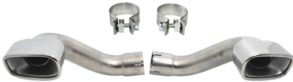
TR-3629 Left & Right S/Steel 304 Slant Cut & Side Slant Cut BMW X5 3.0 E70 2007-2010 "V8 Look" Total Length=350mm Outlet Dimensions=140x75mm Inlet(ID)=66mm
