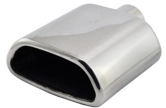
BL183 S/Steel 304 Straight Cut / Double Layer Total Length= 188mm Outlet Dimensions= 159x70mm Inlet(OD)= \Phi 54 -50mm
