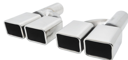
TR-3604 Left & Right S/Steel 304 Straight cut / Double Layer Total Length= 310mm Outlet Dimensions= 190x65mm Inlet(OD)= 64mm
