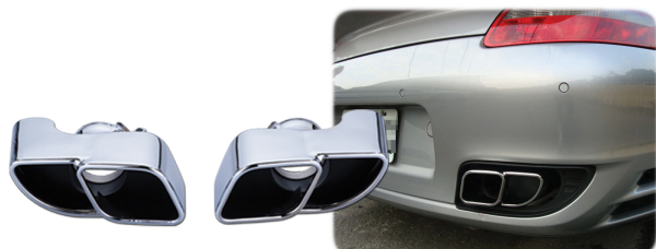
06-8606 Left & Right S/Steel 304 - Chrome plated Porsche 997 non-turbo Carrera S 3.8i (355hp) '04-'08 Porsche 997 non-turbo Carrera S 3.6i (325hp) '05-'08 Porsche 997 non-turbo Carrera 4S 3.8i (355hp) '05-'08 Total Length= 135mm Oval= 185x81mm Inlet(ID)= 60mm
