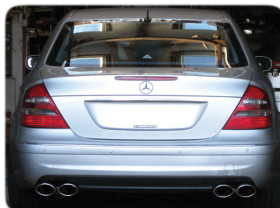
BL222L Left BL222R Right S/Steel 304 Slant Cut / Single Layer "Mercedes AMG" Style Total Length= 200-185 mm Outlet Dimensions= 227x70mm Inlet(OD)= \Phi 60 mm
