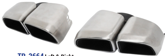
TR-3664 Left & Right S/Steel 304 Slant Cut & Side Slant Cut Porsche Panamera 970 2014-2016 4S Turbo Total Length= 240mm Dimensions= 220x80mm Inlet(ID)= 102x54mm
