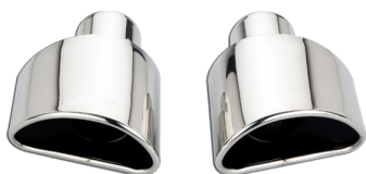
LF165L Left LF165R Right S/Steel 304 Slant Cut & Side Slant Cut Total Length=210mm Outlet Dimensions=145x80 Inlet(OD)= \Phi 64mm
