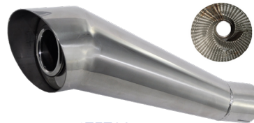
175798 S/Steel 304 "Twister" Perforated pipe Body Length = 300mm Inlet Diameter = 50mm Body Diameter = 100mm
