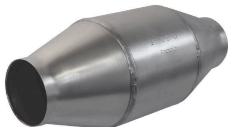
90950182 Inlet=70.5mm Body Diameter=130mm Total length=312mm Metallic substrate 200cps HD (For Porsche and High Performance Cars)
