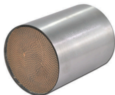
SUB40 Diameter= 100mm Length= 130mm Euro4 / 200cpsci(Cells) High Loading / Premium Quality
