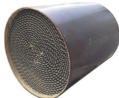
90603102 Diameter= 93mm Length= 130mm 100cpsi(Cells)
