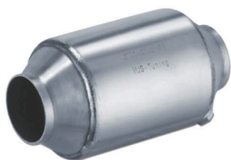
90950140 Inlet=61.5mm Body Diameter=108mm Total length=182mm Metallic substrate 200cps
