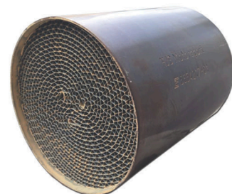
90603105 Diameter= 108mm Length= 130mm 100cpsi(Cells)
