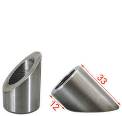
998150 S/Steel Lambda boss with 50dgrs angle M18x1.5 \Phi 25 L=33-12mm
