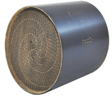
90603444 Diameter= 121mm Length= 112mm 200cpsi(Cells) / Euro5/6 HD (For Porsche and High Performance Cars)
