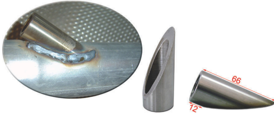
998175 S/Steel Lambda boss with 75dgrs angle M18x1.5 \Phi 25 L=66-12mm
