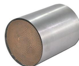
SUB63 Diameter= 130mm Length= 130mm Euro6 / 200cpsci(Cells) High Loading / Premium Quality
