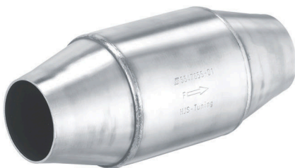
90950082 Inlet=70.5mm Body Diameter=121mm Total length=292mm Metallic substrate 200cps
