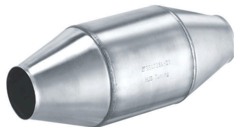
90950070 Inlet=66.6mm Body Diameter=130mm Total length=326mm Metallic substrate 200cps
